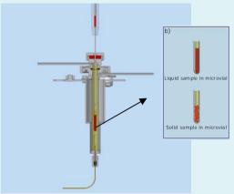
Figure 1: Direct large volume liquid injection of a dirty extract into glass micro vial (b).
