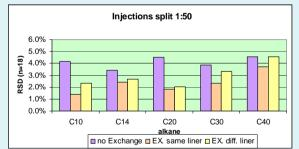
Conditions: alkane mix (12.5 µg/ml); inj.volume 1µl; liner: DMI liner with cup; OPTIC Temp prog.: start 50°C (10 sec.) to 350°C (rate 10°C/s); Flow: start 100 ml/min (before inj.) then split 1:50; column flow: 1ml/min; column: TC5/MS, 0.25mm x 30m (0.25µm film); Oven prog.: 45°C (2 min hold) to 325°C (rate 30°C/min) hold for 11 min.
