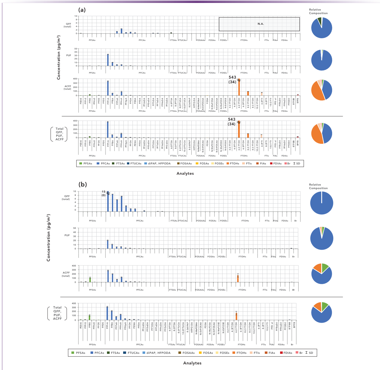
FIGURE 3: Comparison of the two 24-h sampling events. (a) PFAS analyses from the first sampling event ( n = 3 ) with weather: southwest wind; mostly clear/sometimes foggy; 10 to 24 °C (16 °C average); (b) PFAS analyses from the second sampling event ( n = 3 ) with weather: northwest wind; clear; -3 to 11 °C (3 °C average).
