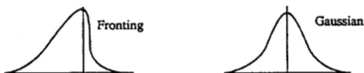
Figure 1.2. Fronting due to overloading of the column.
