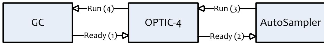
Figure 3.7      OPTIC-4 state diagram in "Master" mode
