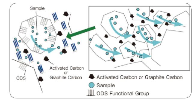
Figure 2. Adsorption on MMSE.
