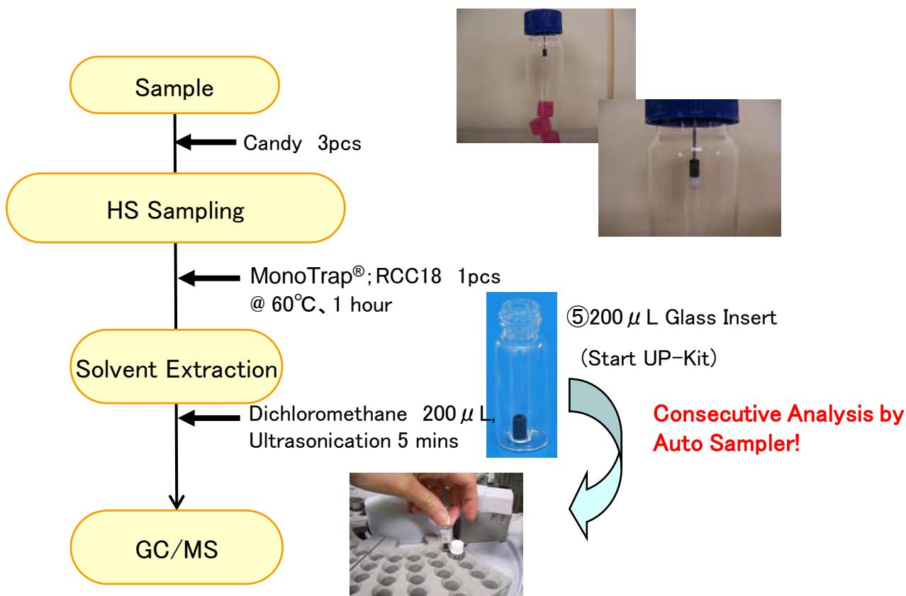
RCC18 and RSC18 can be used with existing auto sampler inert vials to elute without using the MT Extract Cup.
