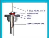
The OPTIC inlet can also be used for on-column injections. GL Sciences has designed a tool that enables true on-column injection using OPTIC inlet without an on-column liner. The on-column tool is very easy to install without any press fit connection. The syringe needle (gauge 26) goes really into the retention gap where the injection takes place.
