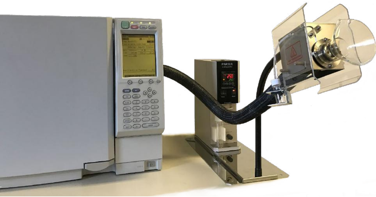
PHASER with 100 cm transfer line and Shimadzu 2010 GC
