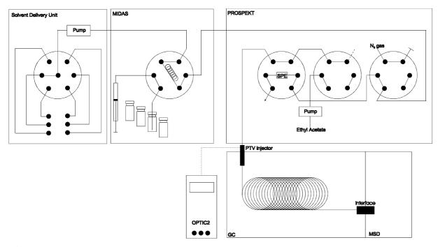
Figure 1. Set-up for on-line SPE–PTV–GC–MS.
