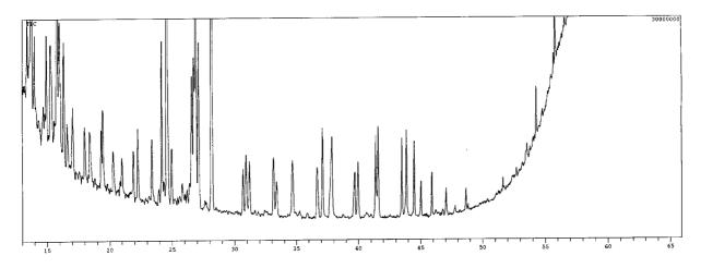
**Figure 6.** On-line SPE–PTV–GC–MS chromatogram of 10 mL of Eindhoven tap water spiked at the level of  $1 \mu g/L$  using correct solvent vent time.
