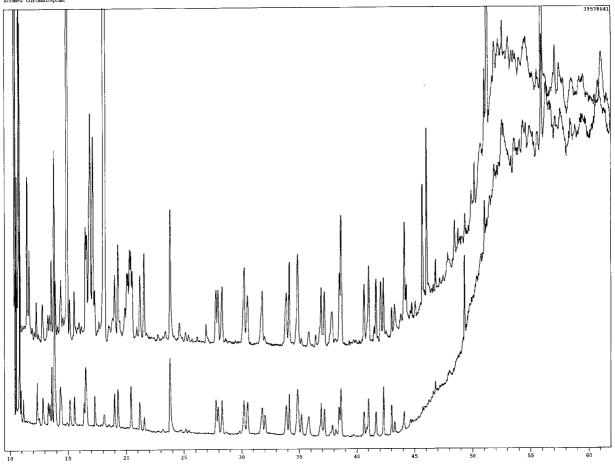
**Figure 3.** Lower chromatogram, 50  $\mu$ l of an 200 g/ $\mu$ l standard; Upper chromatogram, Off-line SPE PTV–GC–MS full scan chromatogram of 10 mL spiked Meuse water at the level of 1  $\mu$ g/l.
