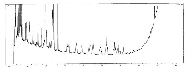
**Figure 5.** On-line SPE–PTV–GC–MS chromatogram of 10 mL of Eindhoven tap water spiked at the level of  $1 \mu g/L$  using a too short solvent vent time.
