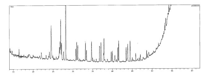
**Figure 4:** On-line SPE–PTV–GC–MS chromatogram of 10 mL of Eindhoven tap water spiked at the level of 1 µg/L using a too long solvent vent time.
