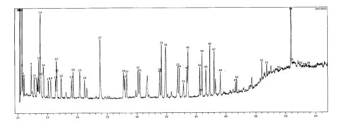
**Figure 2.** Full scan chromatogram of 50  $\mu$ l of an ethyl acetate standard mixture at the level of 200 pg/ $\mu$ L.
