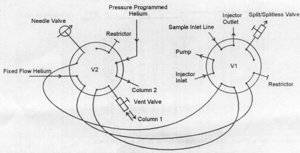
Interface set in sample acquire/secondary column analysis position.
