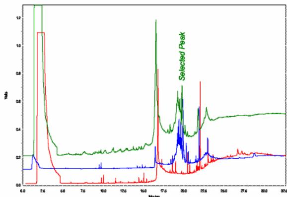
**Figure 4:** Comparison of the analysis of 5000 ppm mineral oil in sunflower oil with (middle) and without (top) selective exclusion and pure sunflower oil (bottom)
