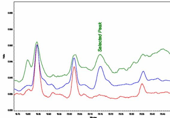
**Figure 6:** 5 ppm mineral oil in sunflower oil with (middle) and without (top) selective exclusion compared to pure sunflower oil (bottom)
