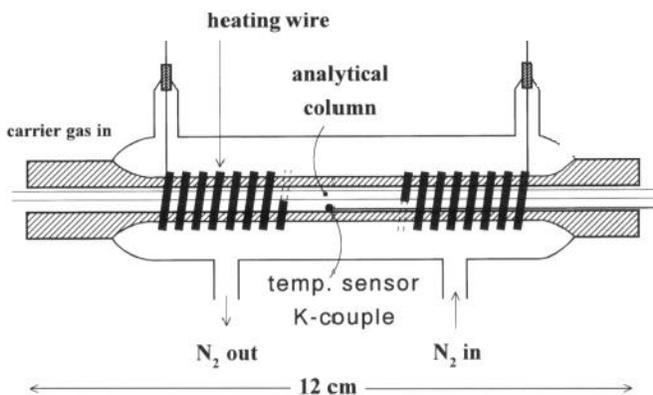
**Figure 2.** Schematic representation of the cold trap.
