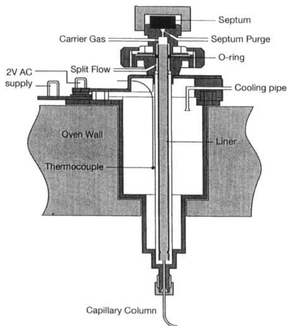
**Figure 1.** The OPTIC 600 PTV injector
