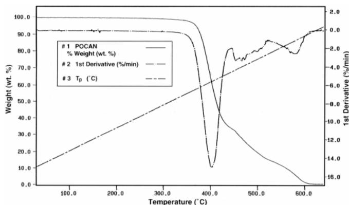
**Figure 3.** TGA-plot of the polycarbonate-polybutadieneterephthalate blend. The first upper curve is the loss of weight (%), the second is the first derivative of the loss of weight and the third is the linear temperature program.
