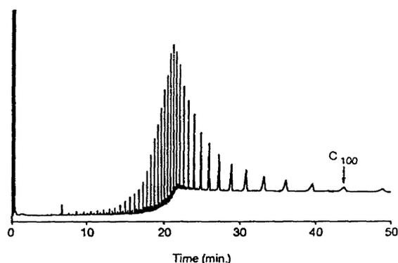
Figure 5. HT-GC separation of Polywax 1000. GC temperature programme started at 75 °C.
