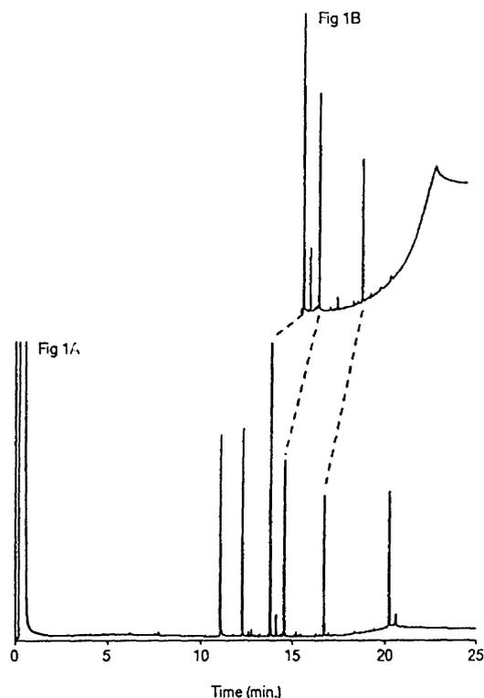
Figure 1. Analysis of polymer additive mixture. Influence of PTV final temperature: A: Final PTV temperature 599 °C. B(insert): final PTV temperature = 400 °C. Components in elution order: Cyasorb 531, Tinuvin 770, Irganox 1076, Tinuvin 144, DSTDP, Irganox 1010.
