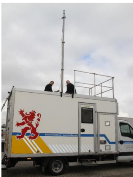
Mobile lab for in situ VOC analysis.
